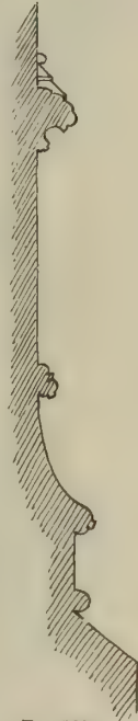
FIG. 1091. The Collegiate Church of Rosslyn. Base Mouldings and Lower String Course, with Peculiar Mould- ing above the latter.
